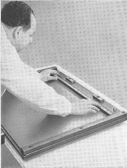
Illus. 131: Inserting the head locking bar which is provided with a scale and pin holes for the transparent sheet.
