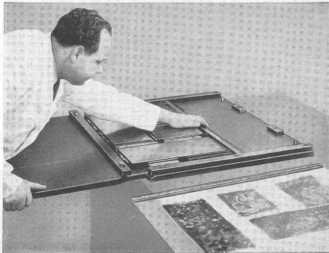
Illus. 135: After loosening the rear locking bar the forme locked between the bearers is slid on to the imposing board and thus can be taken to the machine.
