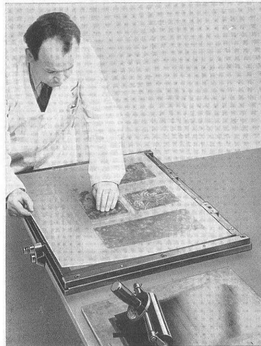
Illustration 128: After the forme has been inked the transparent sheet is folded down and an image is obtained by rubbing heavily over the foil.
