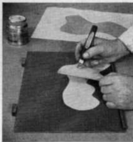
Makeready is pasted under the die-cutting plate.
